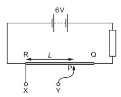
Terminal X is connected to fixed point R. Terminal Y is connected to point P, a connection that may be made at any position along the wire. *L* is the distance between R and P.
