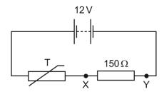
What is the resistance of T when the alarm is triggered?
