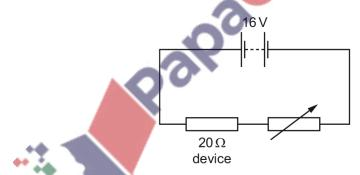
What is the resistance of the variable resistor when the power dissipated in the electrical device is 4.0 W?
