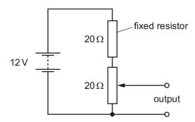
The fixed resistor and the potentiometer each have resistance  $20\Omega$ . The circuit is designed to provide a variable output voltage.
