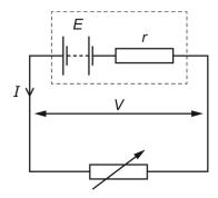
The variable resistor is adjusted so that I increases.
