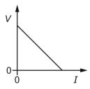
As the cell reaches the end of its useful life, its internal resistance increases and its electromotive force (e.m.f.) decreases.
