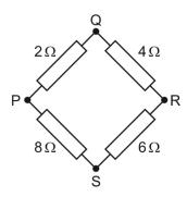
The resistance may be measured between any two junctions.
