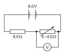
What is the range of the voltmeter reading?
