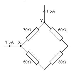
What is the current in the resistor of resistance  $30 \Omega$ ?
