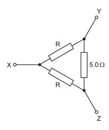
The resistance between Y and Z is found to be  $2.5 \Omega$ .
