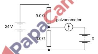
The galvanometer has a current reading of zero.
